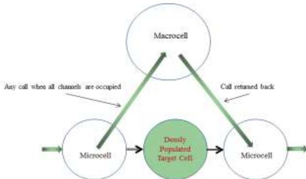
Figure2. Traffic management by skipping the occupied target cell
