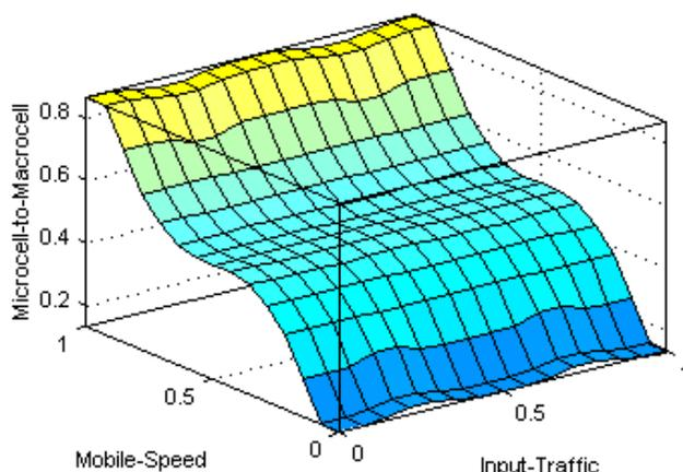
Figure7. Microcell to macrocell handoff with Input traffic and Mobile speed
