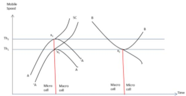
Figure1. Mobility of mobile station from Microcell to Macrocell and vice versa
