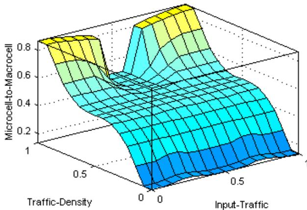
Figure6. Microcell to macrocell handoff with Input traffic and traffic density
