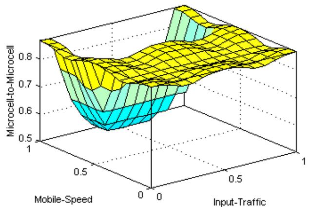
Figure5. Microcell to microcell handoff with Input traffic and Mobile speed
