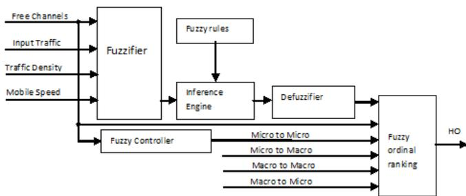
Figure3. Block diagram describing fuzzy control for handoff
