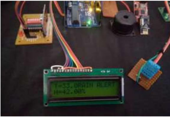
Figure 13: The 2x16 LCD shows that a rain alert using DHT11 sensors.
