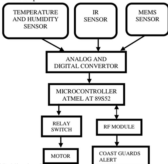
Figure 1: Block diagram of Receiver setup in the boat
