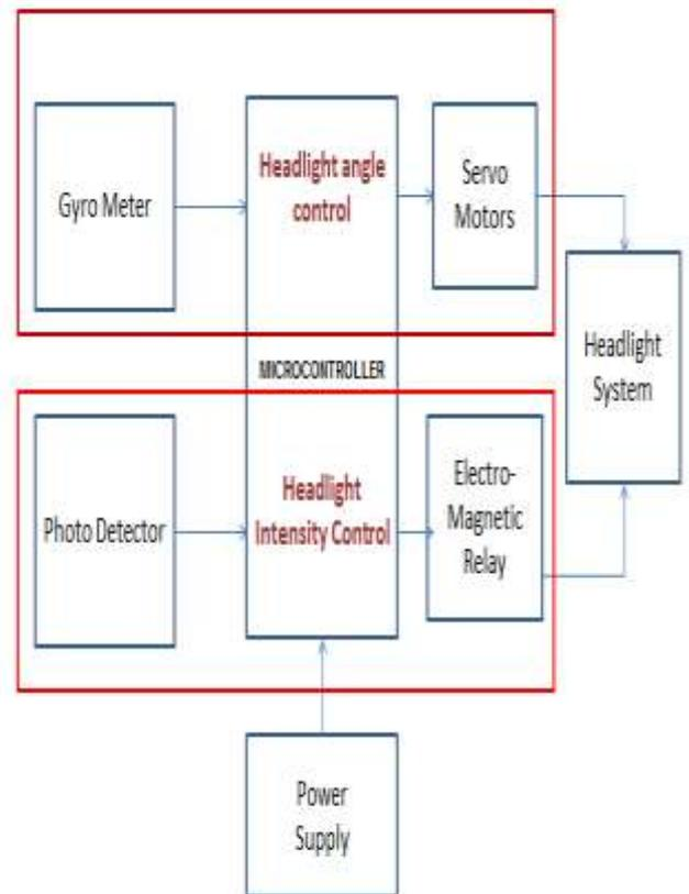
Figure 7: Overall Block Diagram
