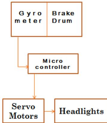
Figure 5: Headlight Angle Control
