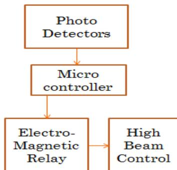
Figure 6: Headlight Intensity Control
