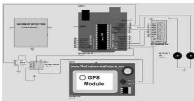
Figure.9Circuit diagram of Accident detection system in vehicle
