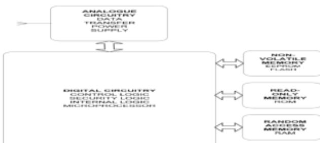
Figure 2. Basic Structure of an RFID transponder
