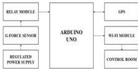
Figure 11. Accident detection system in vehicle
