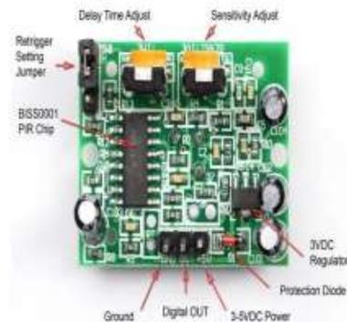
**Fig 4 PIR Motion Sensor**
