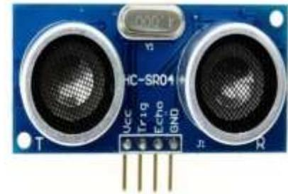
**Fig 3 Ultrasonic Sensor**
